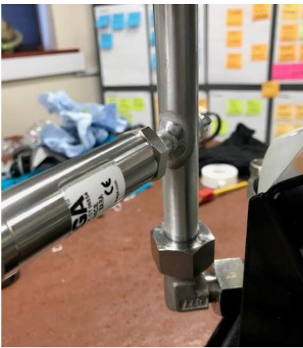
Figure 2: Omega Pressure Transducer Probe
