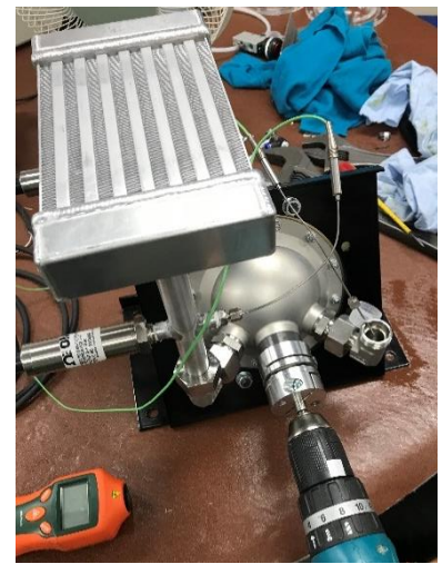
Figure 4: Heat Exchanger/Test layout
