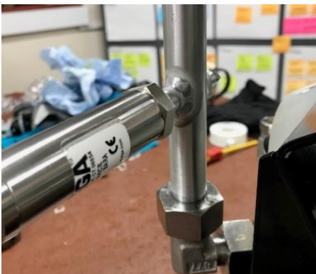
Figure 12: Omega Pressure Transducer Probe
